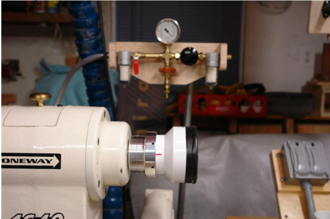
After putting it all together, I tried the system with a piece of 3/4" Maple board held to a 3" vacuum chuck and the system was drawing 25.5 inches of mercury. Given that the pump alone is rated to pull ~26 inches of mercury, it seems that I have little to no leakage and the system should serve me well.
